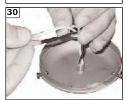
Install keeper nut over lead wires.
